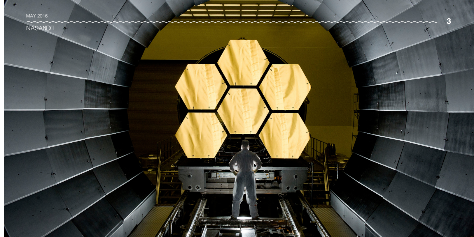
The first six of 18 gold segments that will form NASA's James Webb Space Telescope's primary mirror undergo cryogenic testing. Webb will be the premier observatory for exploring the first luminous glows after the Big Bang and the formation of our own solar system. NASA/MSFC/David Higginbotham
