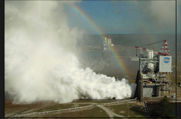
The SLS Program successfully completed a 380 second test of RS-25 Development Engine 0528 at Stennis Space Center 2/22/17.
