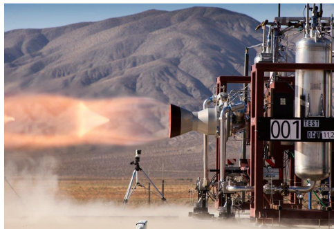
Spacecraft launch abort engine test
