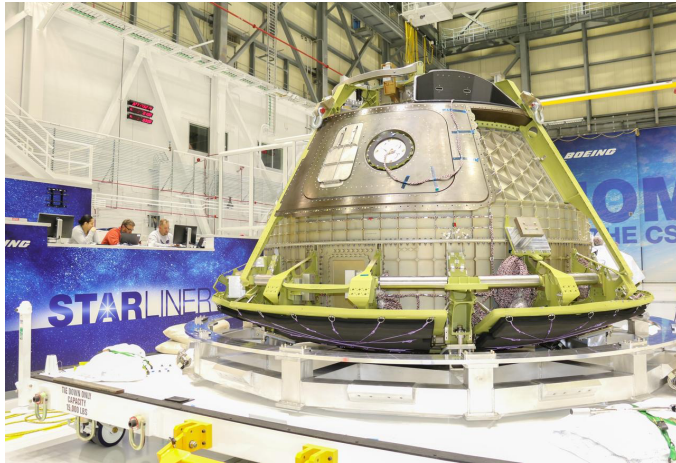
Structural test article completed in the company's facility at NASA's Kennedy Space Center
