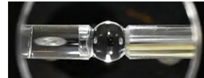
Studying fuel droplet in the high-speed rainbow schlieren deflectometry (RSD) apparatus which can operate at up to 2000 Hz
