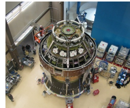
CM and ESM Structural Test in Denver
