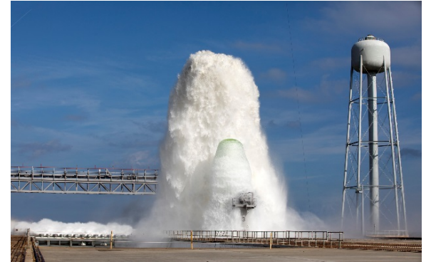
Ignition Overpressure/Sound Suppression System Wet Flow Test at Launch Pad 39B
