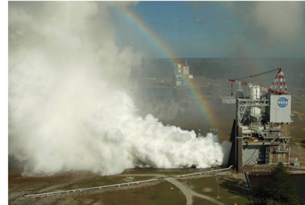
RPT continues to support SLS RS-25 engine testing on the A-1 test stand at Stennis Space Center in Mississippi
