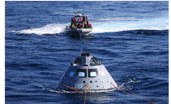
KSC's NASA Recovery Team and the U.S. Navy pull the Orion test article in by a winch line USS Anchorage's well deck during Underway Recovery Test 6
