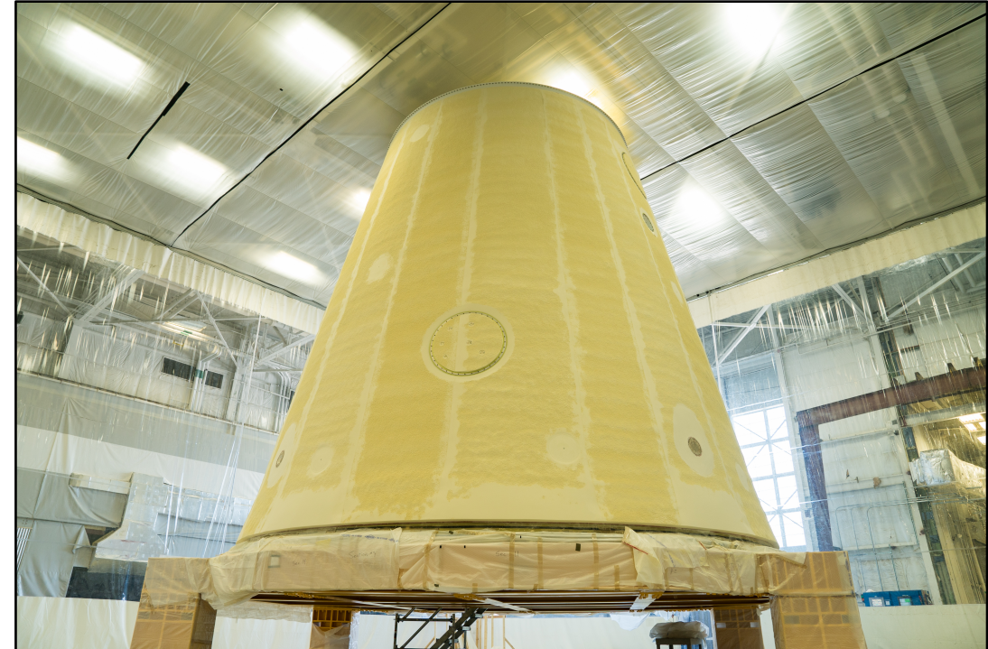
Thermal Insulation Application Complete on LVSA
