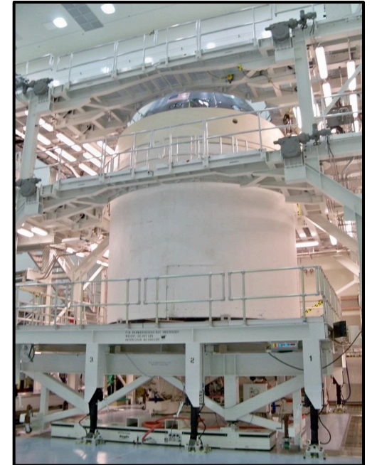
Crew/Service Module Mock-up and Orion Transporter Pallet in the Servicing Stand
