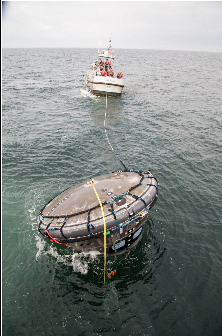
Test of Orion's crew module uprighting system off the coast of North Carolina
