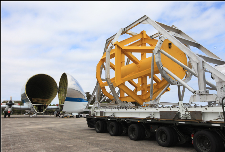
NASA Guppy aircraft modified to fit the Orion crew module and service module stack
