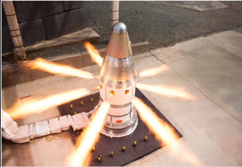
Attitude Control Motor Test Firing
