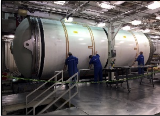
Artemis 2A Forward Motor Segment Thermal Protection System Installation
