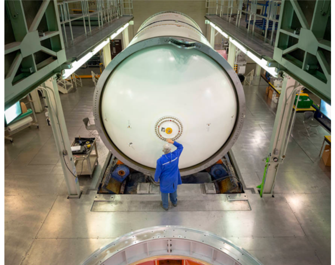
NASA and Northrop Grumman technicians in Promontory, Utah, completed casting, or filling with propellant, all 10 of the booster motor segments for the second flight of NASA's Space Launch System rocket.
