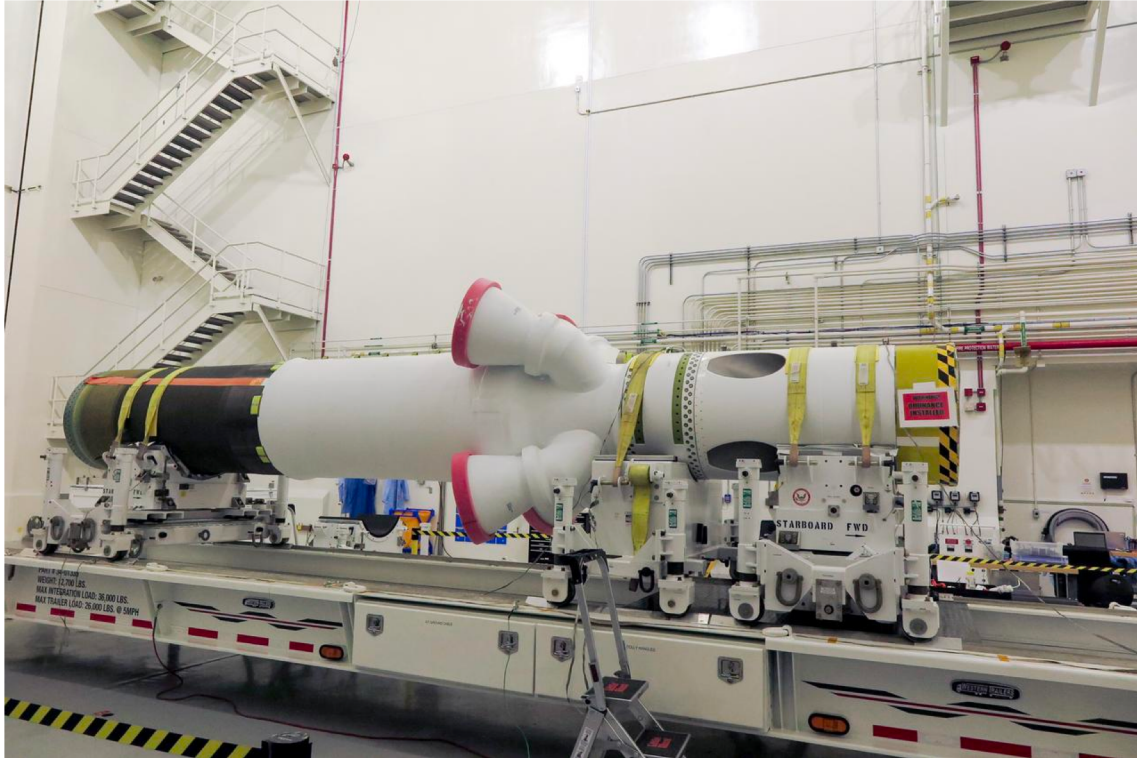
April 2020 - The launch abort motor was integrated with the jettison motor for Orion's launch abort system for Artemis II, inside the Launch Abort System Facility at NASA's Kennedy Space Center.
