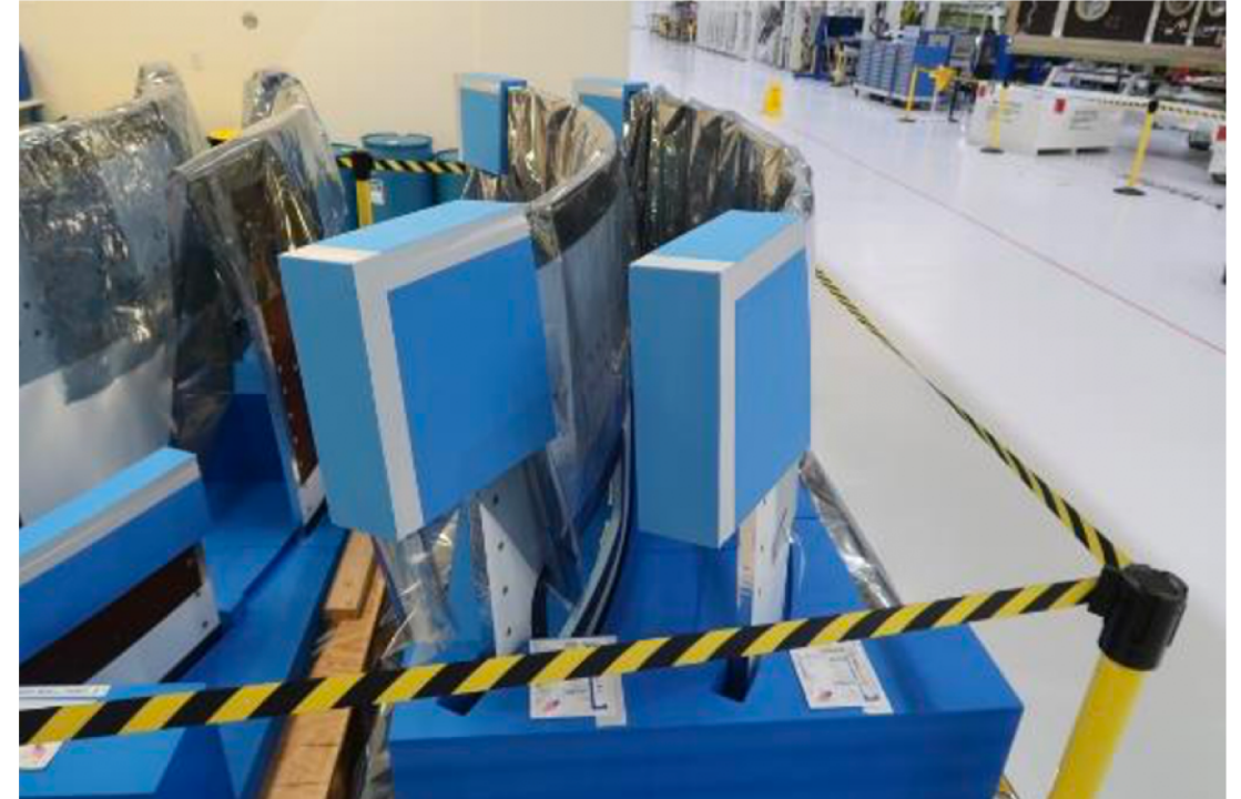
April 2020 - Artemis II crew module adapter outboard walls are in work at NASA's Kennedy Space Center.
