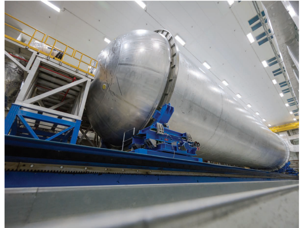
The liquid hydrogen tank for the third SLS core stage is in production at Michoud Assembly Facility.
