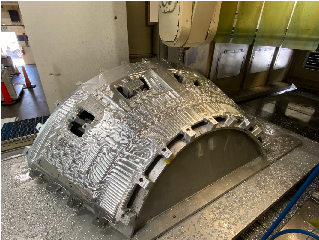
April 2020 - A large aluminum alloy panel for the Artemis III Orion spacecraft is being manufactured by AMRO Fabricating Corporation. The cone panel is one of three segments that make up the upper half of the pressure vessel capsule of the spacecraft.
