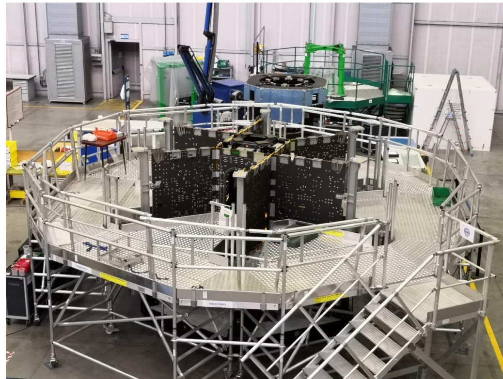
Artemis III European Space Module being assembled at TASI in Turin, Italy
