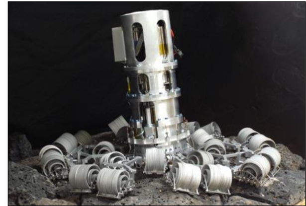
Microspine gripper development at JPL
