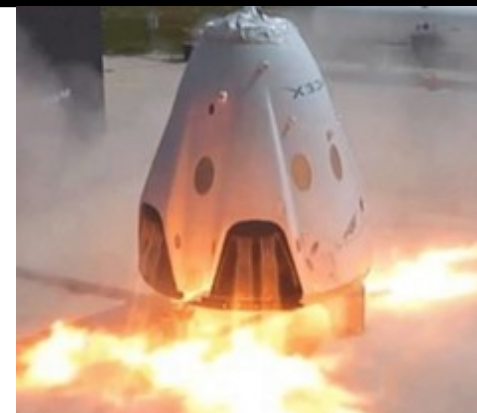
Propulsive Landing Testing
