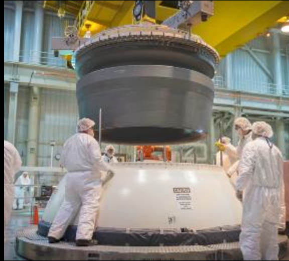
Nozzle installation into the aft booster segment for QM 2
