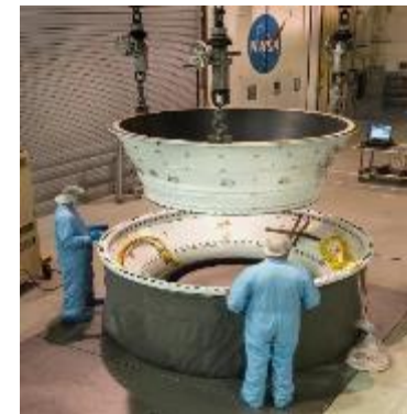
Installation of Forward Exit Cone into Nozzle Assembly
