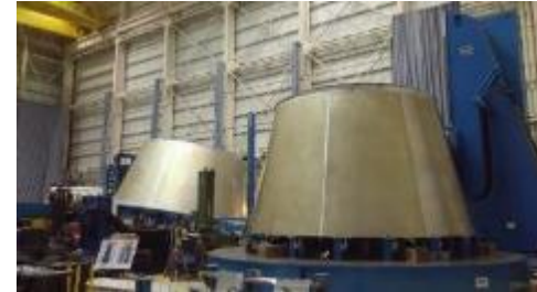
LVSA Structural Test Article Forward & Aft Cones
