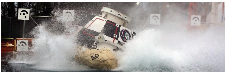
Air Bags Qualification Tested for Emergency Water Landings
