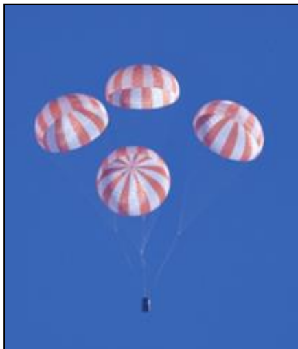
Parachute Mass simulator test
