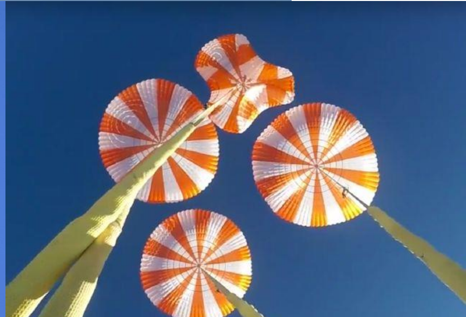
January 27, 2016. Parachute drop test for SpaceX crew Dragon involving four red and white parachutes unfurled from a mass simulator high above the desert near Coolidge, Arizona.
