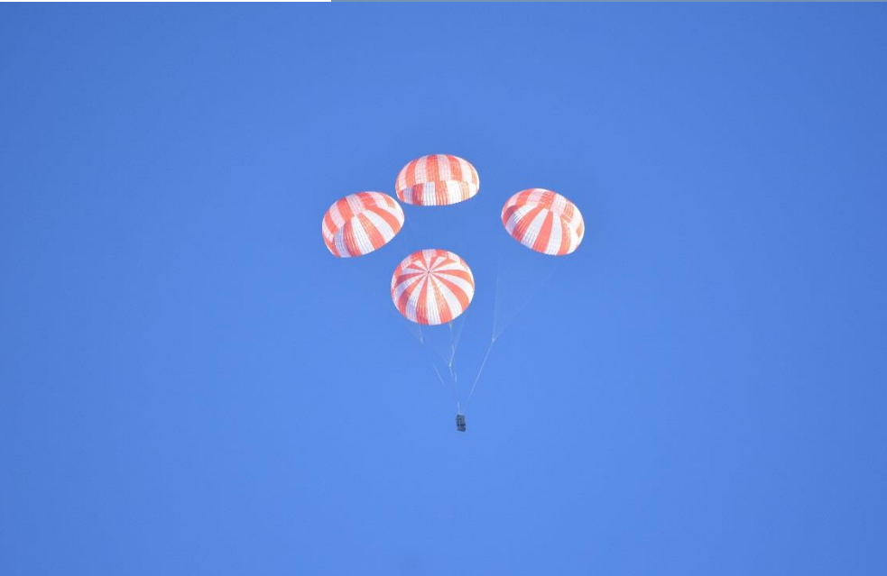
January 27, 2016. Parachute drop test for SpaceX crew Dragon involving four red and white parachutes unfurled from a mass simulator high above the desert near Coolidge, Arizona.
