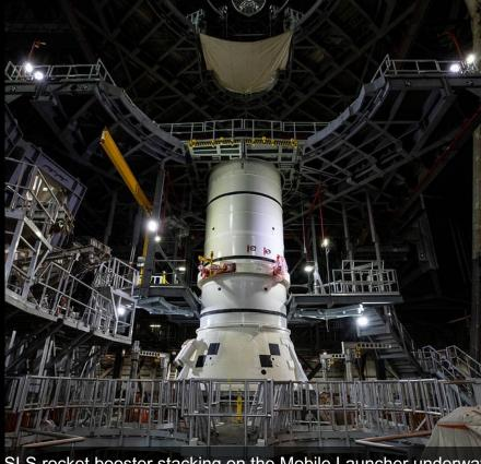
SLS rocket booster stacking on the Mobile Launcher underway in the VAB
