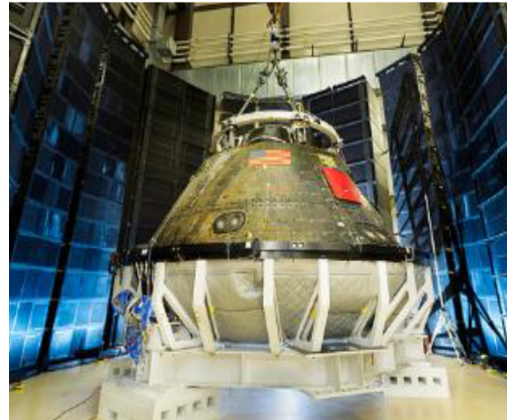
EFT1 Crew Module acoustic testing at Lockheed Martin in Littleton, Colorado
