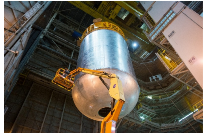
Liquid Oxygen Tank STA completed vertical welds
