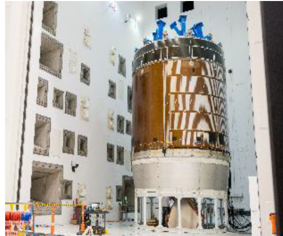
European Service Module Structural Test Article (ESM STA) completes acoustic testing Glenn Research Center Plum Brook Station in Ohio
