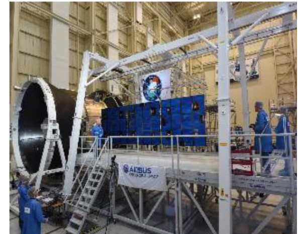
ESM STA solar panel array deployment test at Glenn Research Center Plum Brook Station in Ohio
