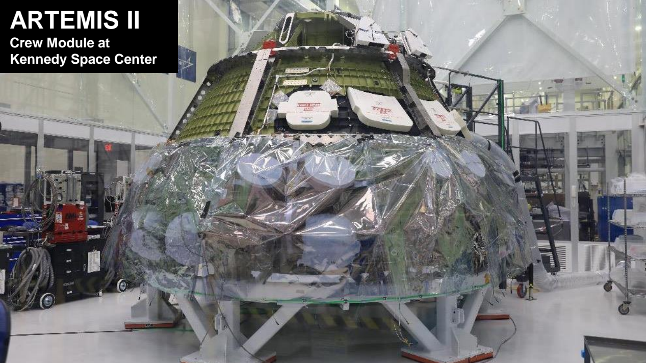
ARTEMIS II Heat Shield at Kennedy Space Center
