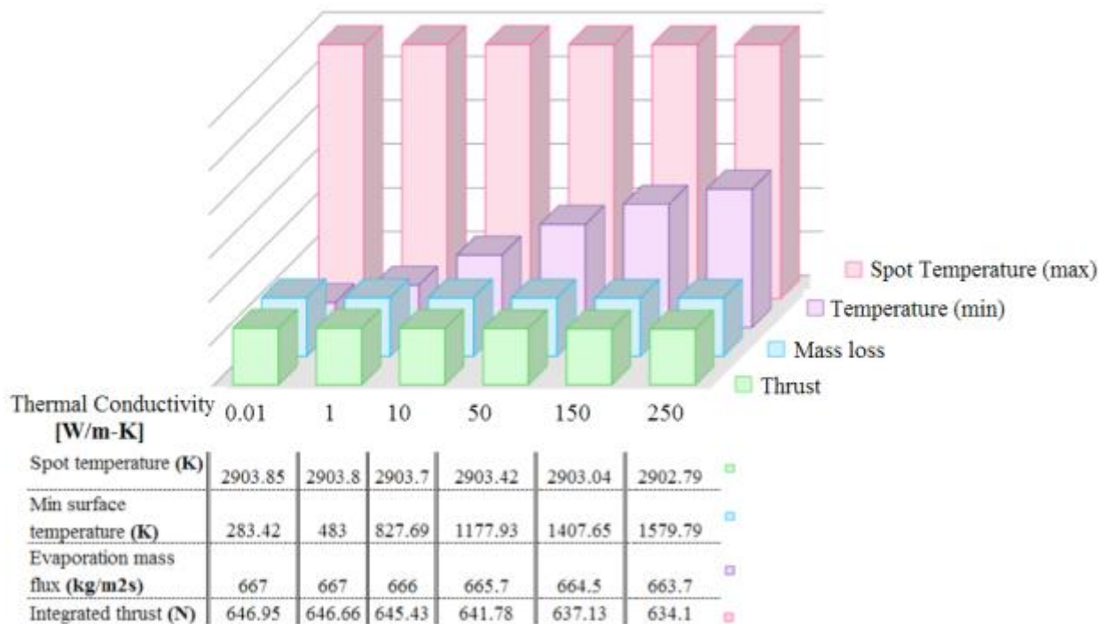
Figure 5-12: Extreme values inputs of thermal conductivity set to 0.01-250 W/m K for SiO 2 – Using 1 MW laser power, spot diameter is 60 mm, with sigma 10 mm, in this case for a 2 m diameter asteroid.
