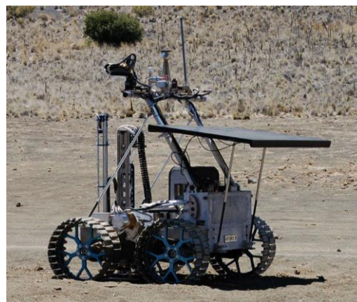
Figure 27. Resolve drill operations on Artemis Jr. rover
