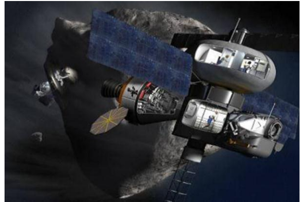
Figure 2: DSH with one MMSEV remaining attached (right), while a second explores at NEA surface (left). MPCV also shown (center).
