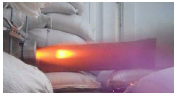
Figure 5. The Electrically Controlled Extinguishable Solid Propellant project is developing a thruster that would allow NASA to demonstrate an innovative throttleable solid rocket motor.
