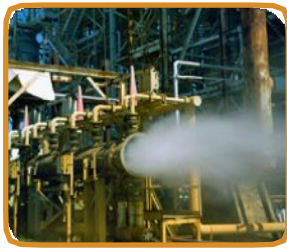
Thermal Protection System Material Test at the Hot Gas Test Facility.
