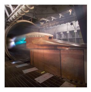
tested the National Aerospace Plane Concept Demonstration Engine, the X43 Hyper-X engine, the Office of Naval Research HyFly Dual Combustor Ramjet Engine, the X43C program's Ground Demonstrator Engine No. 2, and the Air Force Research Laboratory SJX61–1 and SJX61–2 engines. The facility has an array of test support systems that include hydrogen system, silane system, JP–7 and JP–10 systems, ethylene system, model hydraulic system, water cooling systems, and nitrogen purge systems.
