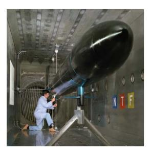
semispan testing with a wide range of instrumentation and measurement techniques.
