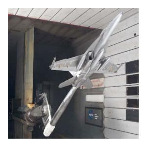
Interchangeability of models among the UPWT test sections allows testing across a wide range of conditions.
