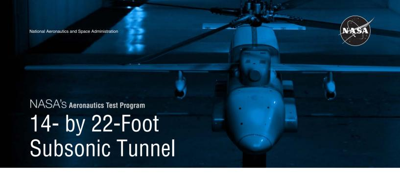
Initially named the V/STOL (vertical/short takeoff and landing) Tunnel, then the 4- by 7-Meter Tunnel, and finally, the 14- by 22-Foot Subsonic Tunnel (14×22) was constructed in 1970 to provide an improved understanding of the aerodynamics of V/STOL aircraft. Studies concentrated on the strong downwash generated by the V/STOL model-lift fans or jets and the interaction of the boundary layer with the vertical or forward-facing, propulsion-flow components.
