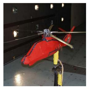
The 14×22 is ideally suited for low-speed tests to determine high-lift stability and control, aerodynamic performance, rotorcraft acoustics, turboprop performance, and basic-wake and flow-field surveys.
