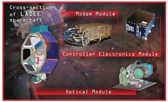
the LADEE spacecraft, is the brain of the LLST, providing fine, closed-loop pointing-and-tracking control of the optical module to Earth. It also provides the command and telemetry interfaces between the LLST and the LADEE spacecraft.
