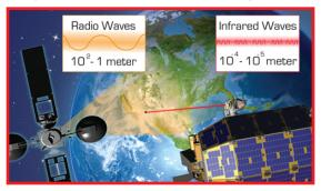
This reduction in antenna size applies for both ground and space receivers, which reduces satellite size and mass. Laser communication terminals can support higher data rates with lower mass, volume and power requirements, a cost savings for future missions. For laser communications to become standard, NASA first must prove the concept is a viable option. NASA's LLCD mission will test this concept.
