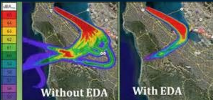
EDA is used to synchronize the descents of all arrival aircraft thereby minimizing fuel consumption, environmental emissions, and noise pollution
