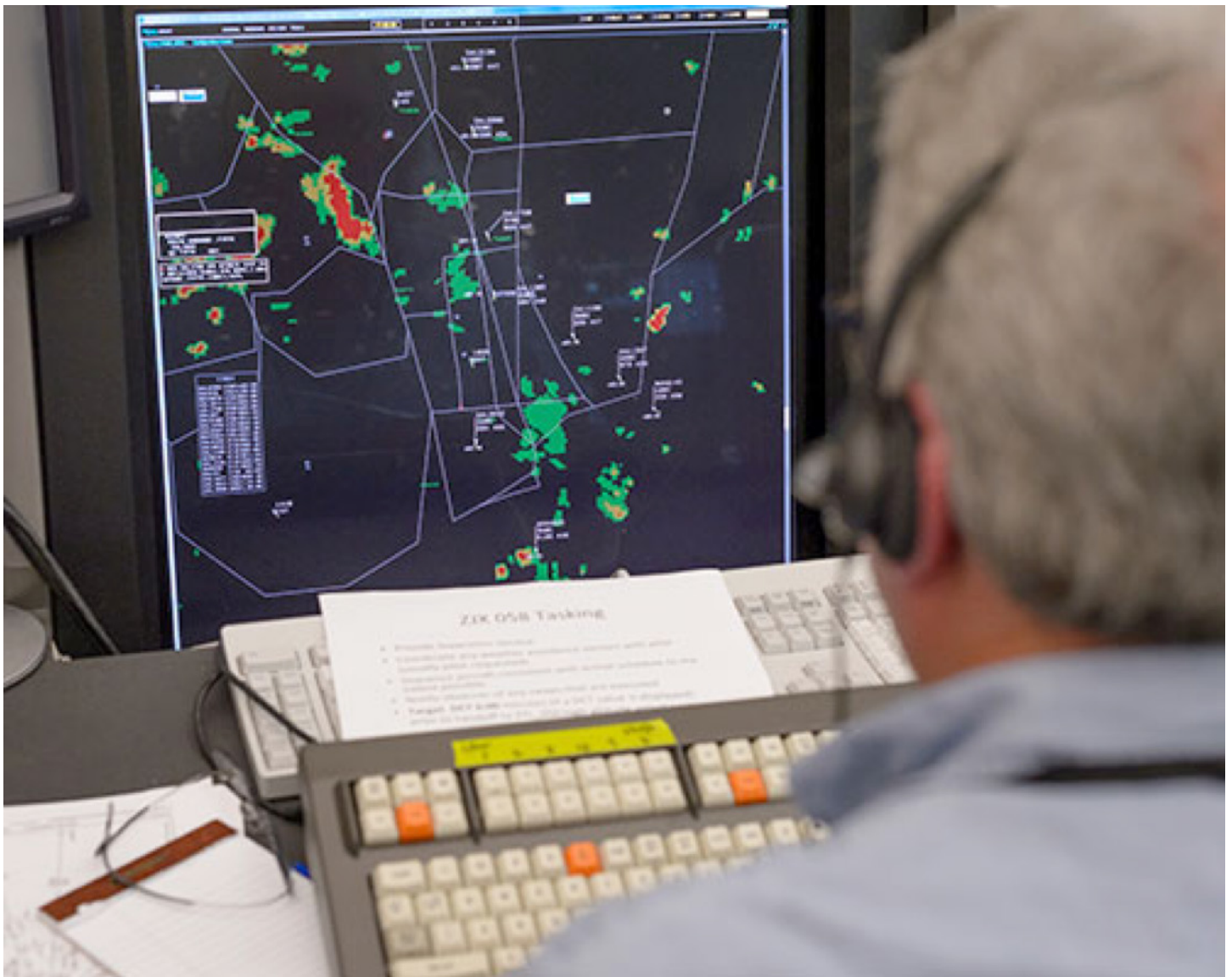
Subject controller using the DRAW tool during HITL simulation #4.
