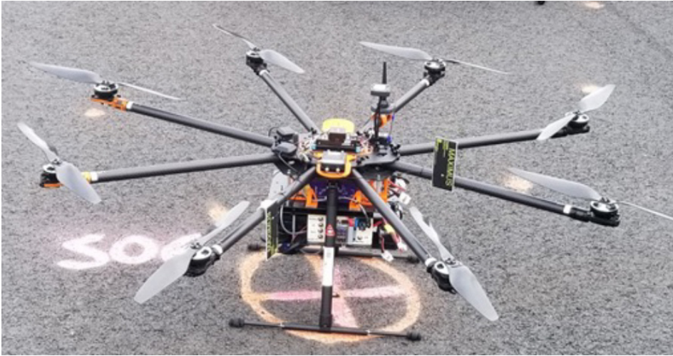
SWS-21 Test Vehicle (Tarot T18 Octocopter)
