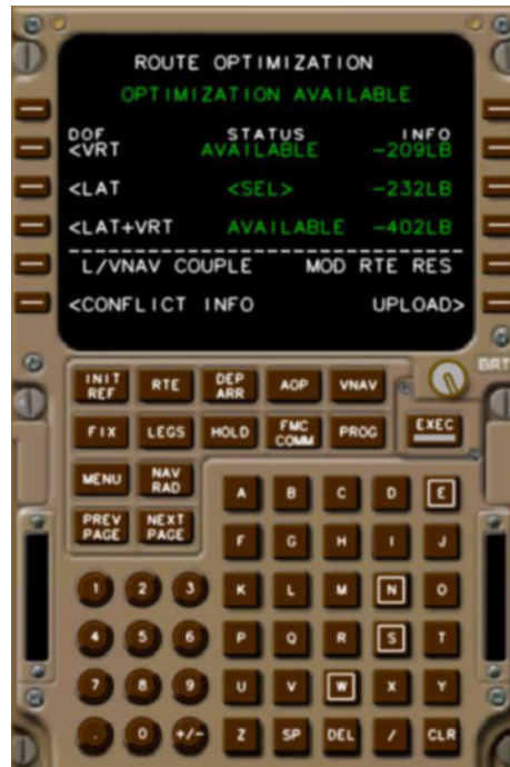
Optimized Trajectory Solutions shown on multi-purpose control and display unit autonomous operations planner page
