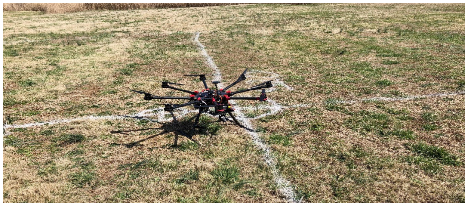
Test of Safe2Ditch ability to find a safe landing spot and effectively land the small UAS.
