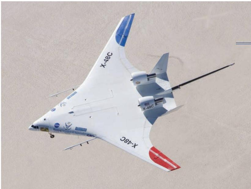
The sub-scale experimental X-48C Hybrid Wing Body flies over Rogers Dry Lake in California. The X-48C is a modification of NASA's X-48B blended wing body aircraft modified to evaluate the low-speed stability and control of a low-noise version of a hybrid-wing-body design. The concepts and technologies being demonstrated through these test aircraft could find their way into all types of new aircraft over the next 20 years, enabling more sustainable, environmentally friendly aviation.
