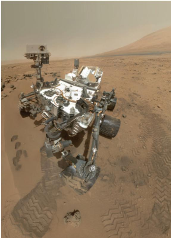
A Curiosity self-image taken by the MAHLI (Mars Hand Lens Imager) camera on the robotic arm. The rover is at Rocknest, having taken several soil samples (bottom left) in Gale Crater, with Mt Sharp in the background. Findings indicate that chemical conditions in Gale Crater were once capable of supporting microbial life. Samples determined that Martian soil contains abundant and easily accessed amounts of water.
