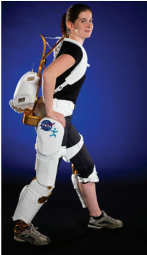
NASA's X-1 Robotic Exoskeleton would help astronauts stay healthier in space with the added benefit of assisting those with physical disabilities here on Earth.
