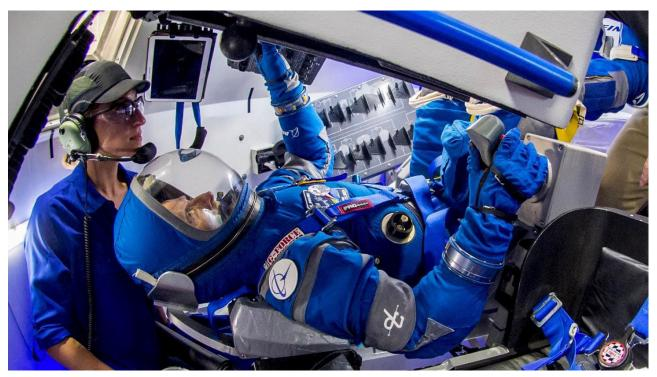
Astronauts heading into orbit aboard Boeing's CST-100 Starliner spacecraft will wear spacesuits that are 40 percent lighter than astronauts wore in years past. Boeing designed the suit with comfort, utility, and production in mind.
