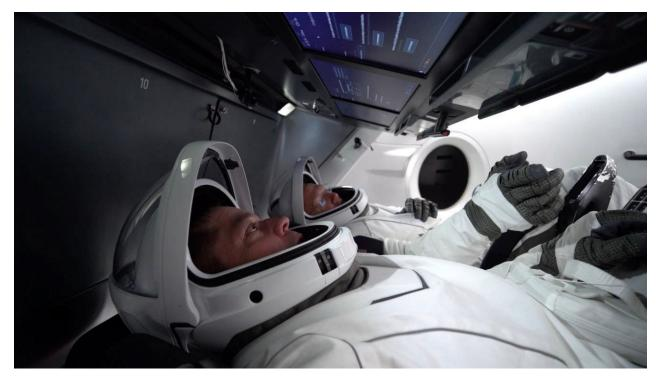
The helmet is custom manufactured using 3D printing technology and includes integrated valves, mechanisms for visor retraction and locking, and microphones within the helmet's structure.
