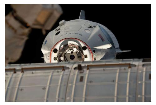
Dragon is composed of two main elements: the capsule, which is designed to carry crew and critical, pressurized cargo, and the trunk, which is an unpressurized service module. The capsule is subdivided into the pressurized section, the service section and the nose cone, which is opened once on orbit and stowed prior to re-entry.
