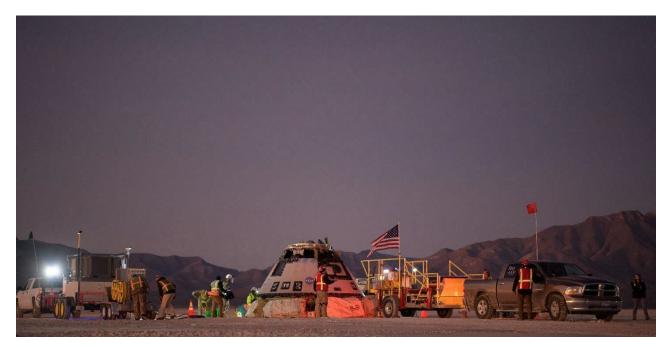
The CST-100 Starliner is designed to land at one of five landing sites in the continental U.S. After re-entering the atmosphere the Starliner will deploy pilot and drogue parachutes, prior to unfurling the spacecraft's three main parachutes. Once the capsule is stable under its parachutes the spacecraft's base heat shield will drop away, allowing the air bag system to inflate prior to a soft landing.
