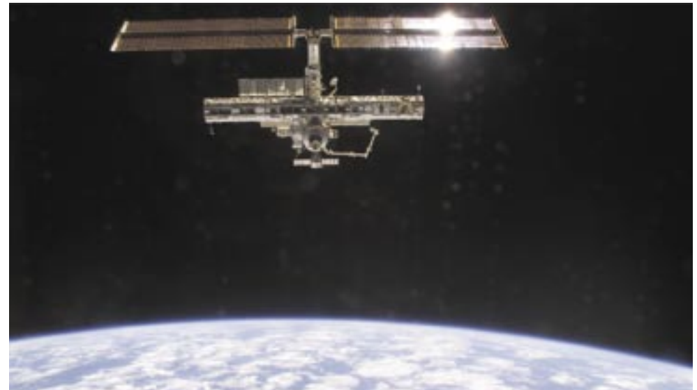
Orbiting 221 miles above the Earth, the International Space Station is seen with the Port One truss and Starboard One truss in place.
