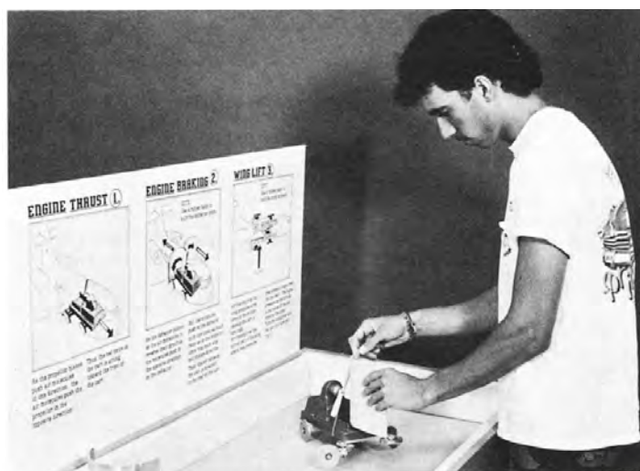
Fig. 2. A rubber band is used to hold the airfoil-shaped wing section in place, allowing the orientation to be changed easily.
