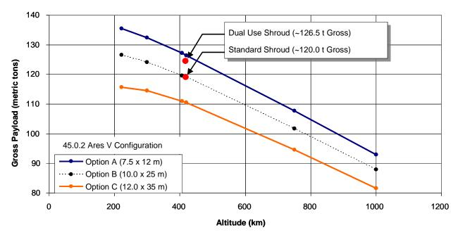
Figure 4-4. Launch vehicle payload performance (45.0.2 configuration).
