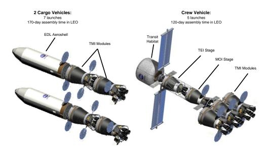
Figure 4-6. Chemical/aerobrake cargo and crewed MTV concepts.
