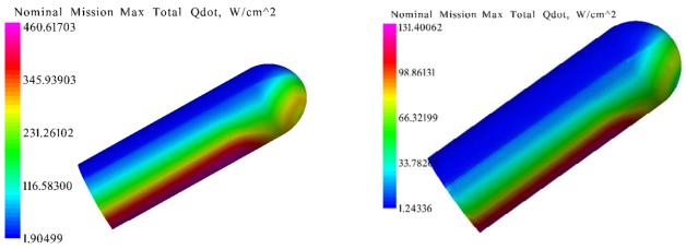
Figure 4-10. Distributed heating rates for the aerocapture and entry phases.
