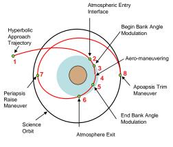
Figure 6-4. Aerocapture flight profile.
