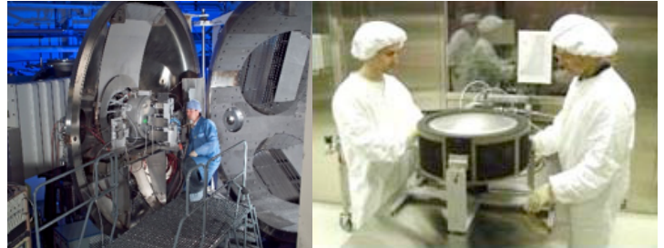
Left: NEXT long-duration test setup. Right: Aerojet prototype NEXT thruster.
