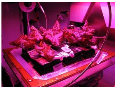
The Plant Pillows growing lettuce during the Veg-01 experiment. "Tokyo Bekana" cabbage is the test crop during Veg-03
