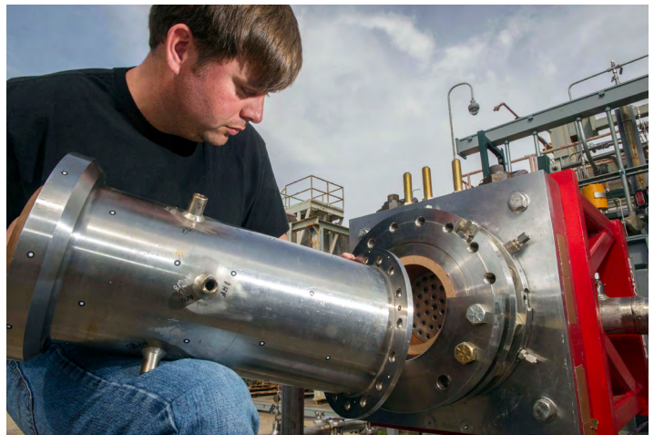
Randall McAllister, a Marshall propulsion technician, installs a complex rocket engine injector made using additive manufacturing or 3-D printing. The tests were performed on Test Stand 116 at the Marshall Center. Testing of various rocket components, such as valves, injectors, and nozzles will improve the design of the future Space Launch System and other spacecraft engines. (NASA/MSFC/Emmett Given)
