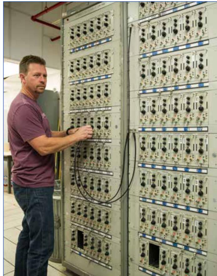
(Bottom left photo) Lockheed Martin Test Operation Contract employee Scotty Herrin checks the status of the A-1 Test Stand accelerometer, which measures rocket engine pump vibrations during a test.
