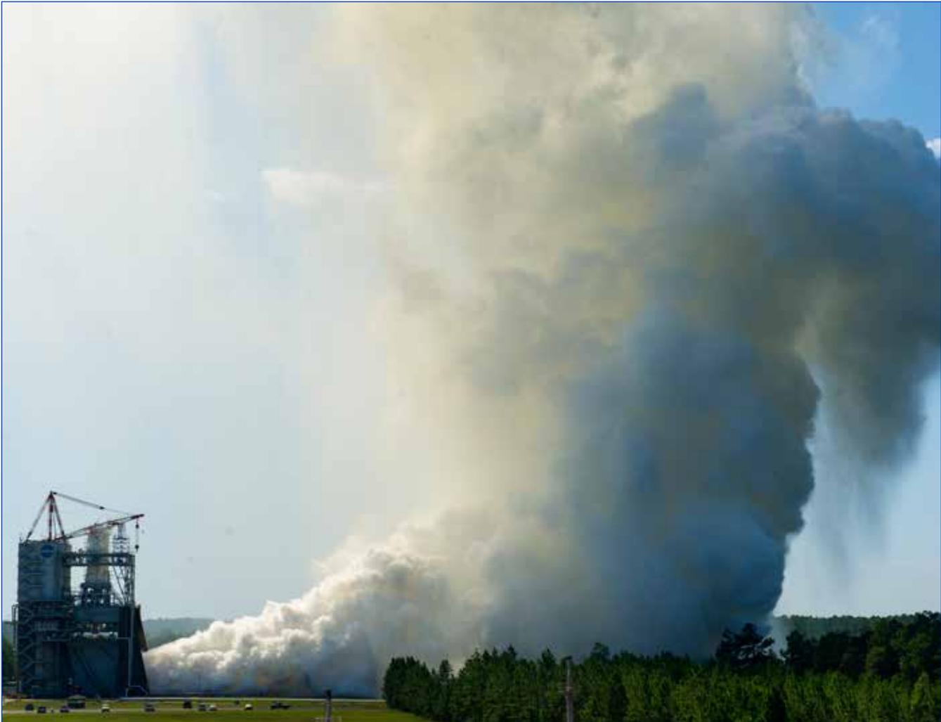
The RS-25 engine fires up for a 535-second test Aug. 27 at Stennis Space Center. This is the final in a series of seven tests for the development
