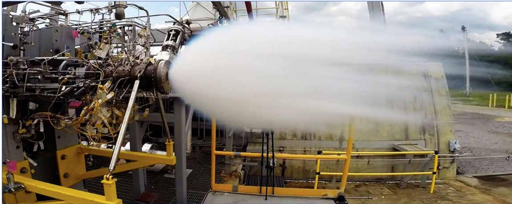
Operators at the E-2 Test Stand at Stennis conduct a test of the oxygen preburner component being developed by SpaceX for its Raptor rocket engine, which is being built to power flights to Mars.
