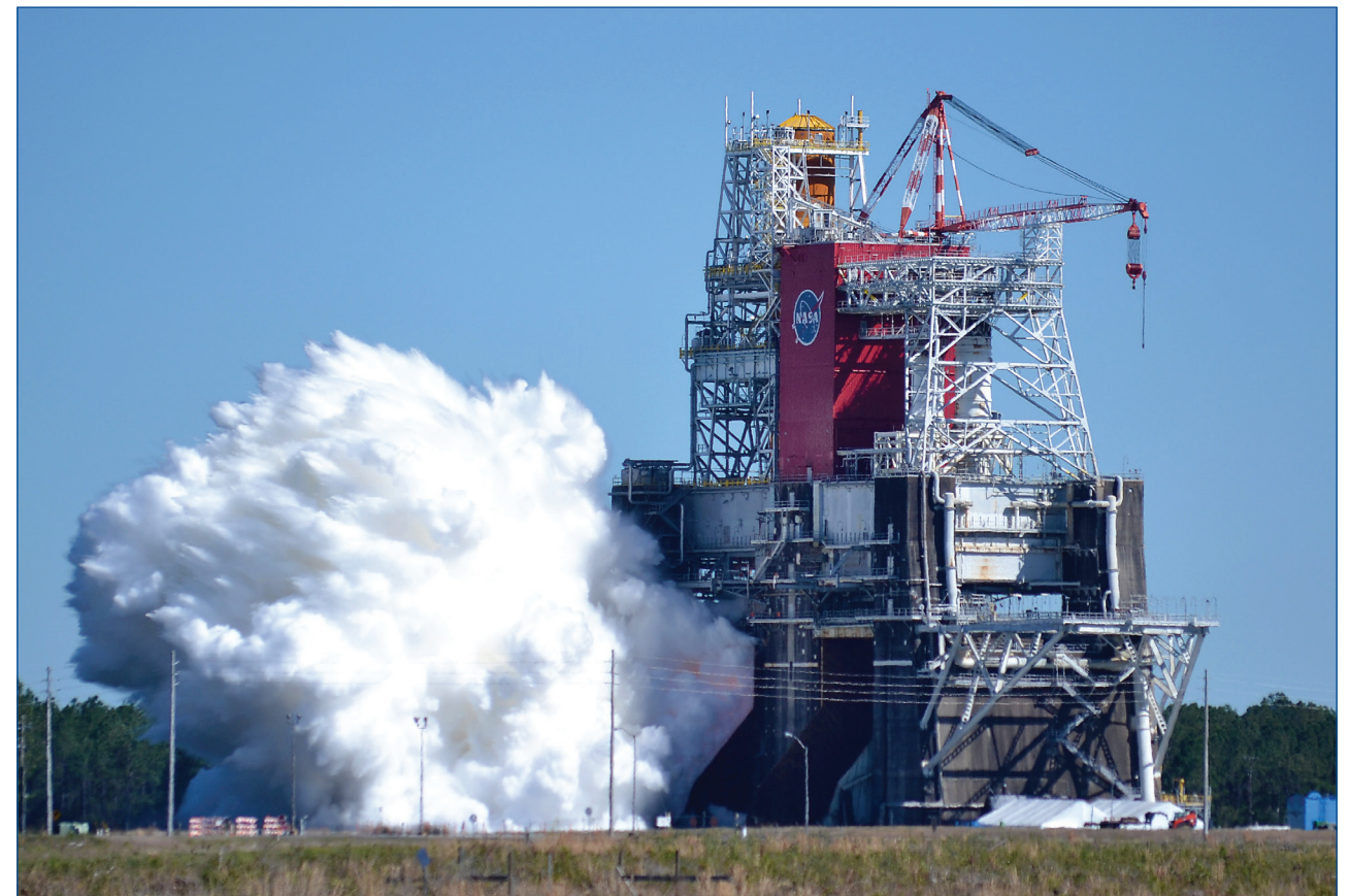
The second Green Run hot fire test begins with a roar as a cloud of water vapor rushes out of the B-2 Test Stand flame deflector bucket.
