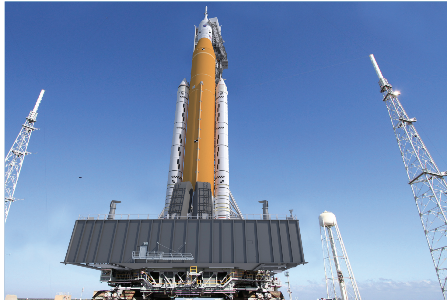
This artist concept shows NASA’s Space Launch System (SLS) rocket on the launch pad. SLS is designed to carry the Orion spacecraft, astronauts as well as important cargo, equipment and science experiments to the Moon, Mars and other destinations. This concept depicts the SLS Block 1 crew configuration that will be used on the Artemis missions to the Moon. NASA is working toward a launch of the Artemis I mission – an uncrewed flight test of the SLS rocket and the Orion spacecraft around the Moon – sometime in the fall of 2021.
