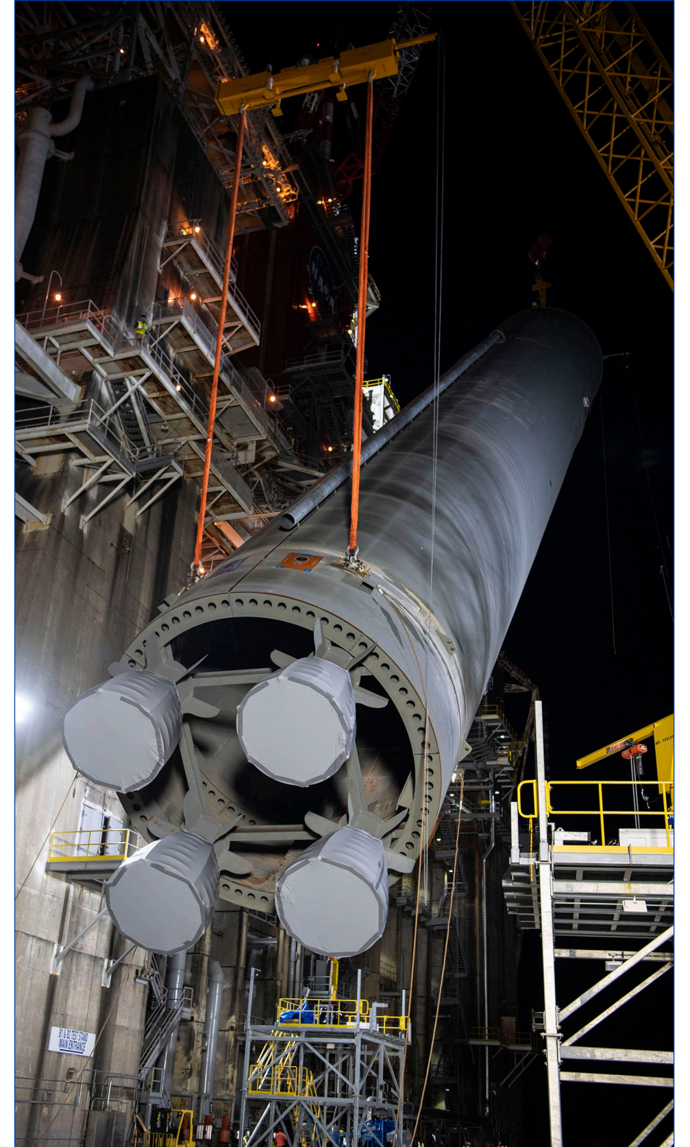
B-2 Test Stand operators perform a lift and installation of the Space Launch System (SLS) core stage pathfinder through the night of Aug. 23-24. The procedure marked yet another milestone as Stennis prepares to install and test the actual core stage that will help power the maiden SLS flight – Artemis I. As photos on this and the following page show, operators used two cranes to lift the pathfinder from its horizontal position, “break” it over into a vertical position and hoist it up and into place on the stand. The exercise allowed operators to practice the procedure and helped confirm the test facility is ready to receive the core stage when it is delivered later this year.
