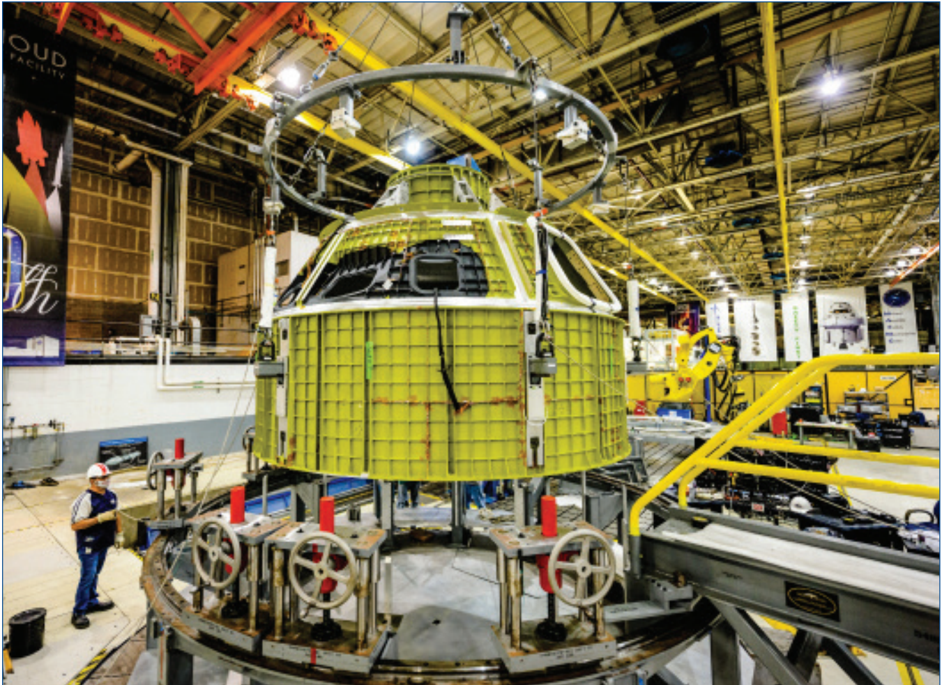
The newly completed Orion pressure vessel for NASA's Artemis III mission is lifted out of the welding tool at Michoud Assembly Facility in New Orleans. Completion of the welding step this month marked a milestone in construction of the Artemis III crew module.
