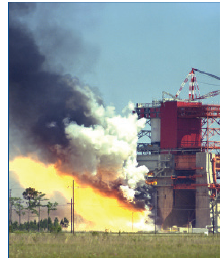
Flames erupt from the B-2 Test Stand flame deflector during a Saturn V S-IC stage test for the Apollo Program.
