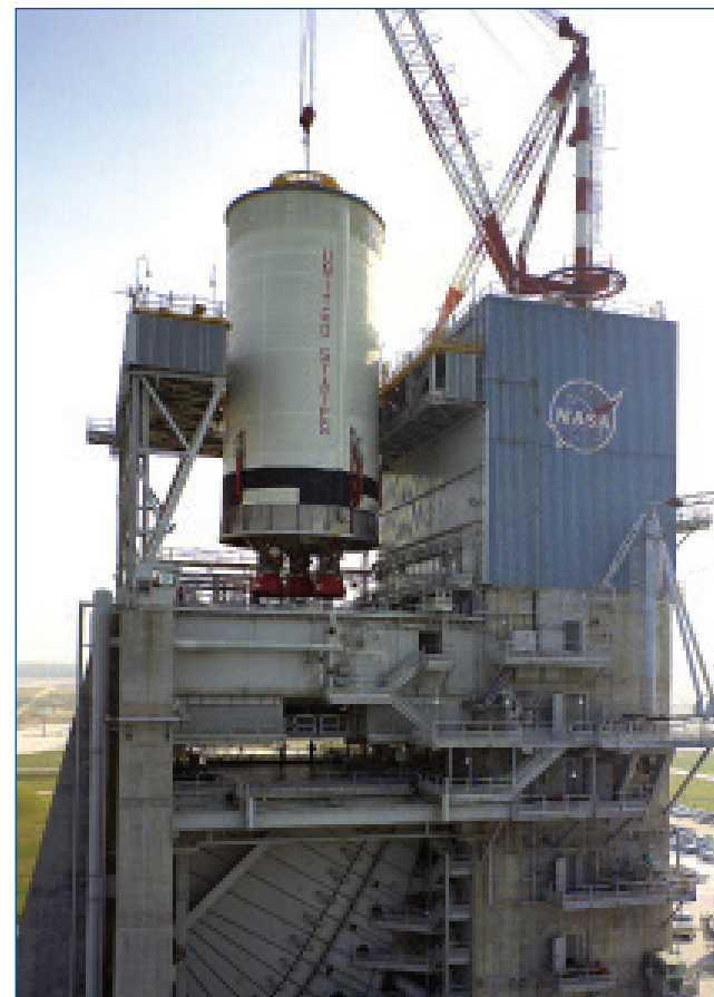
The first Saturn V rocket stage (S-II-T) is lifted onto the A-2 Test Stand at Stennis. NASA conducted the first Saturn V test on site on April 23, 1966.
