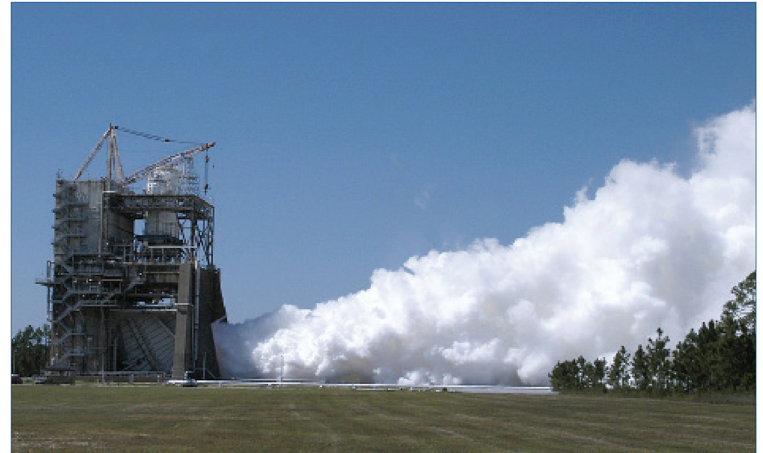
NASA conducts a space shuttle main engine test on the A-1 Test Stand at Stennis. At the base of the stand, the flame deflector directs the engine exhaust horizontally away from the stand. The opening above the flame deflector is where one can glimpse the engine nozzle of the main engine being tested.
