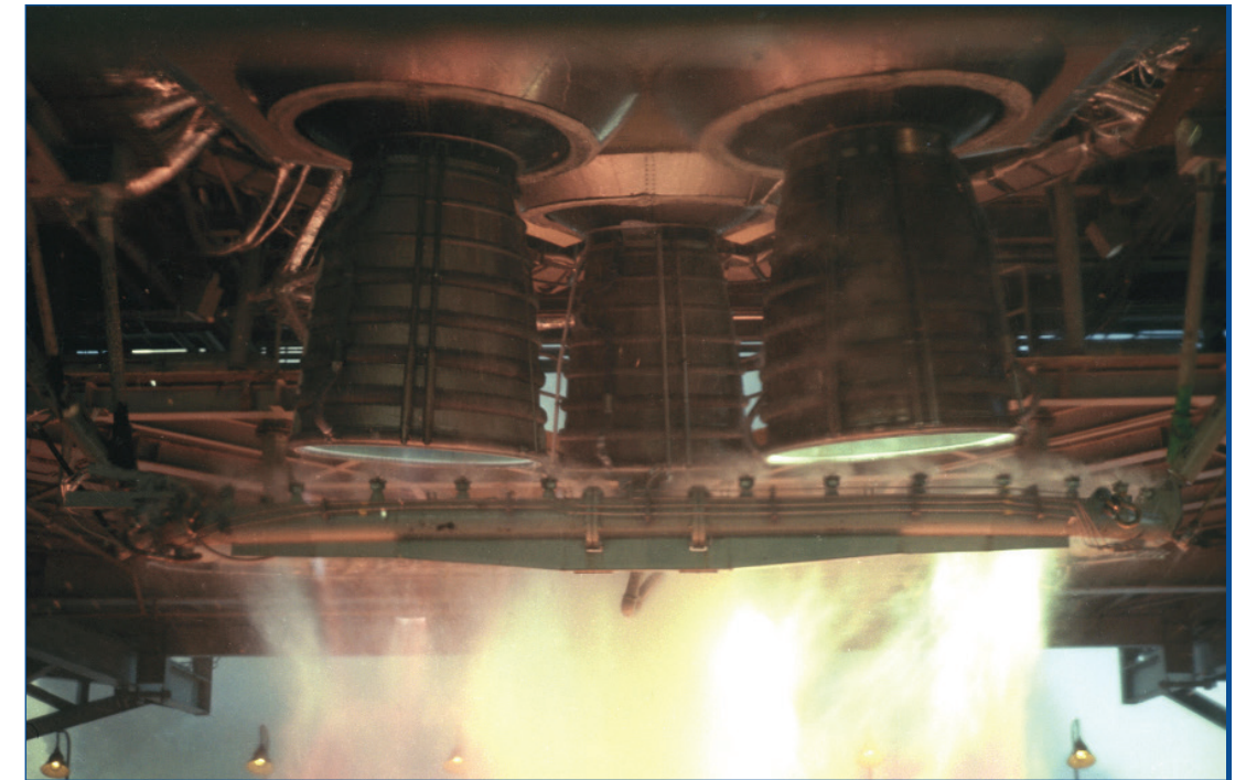
NASA conducts a space shuttle Main Propulsion Test Article hot fire on the B-2 Test Stand between 1978 and 1981..
