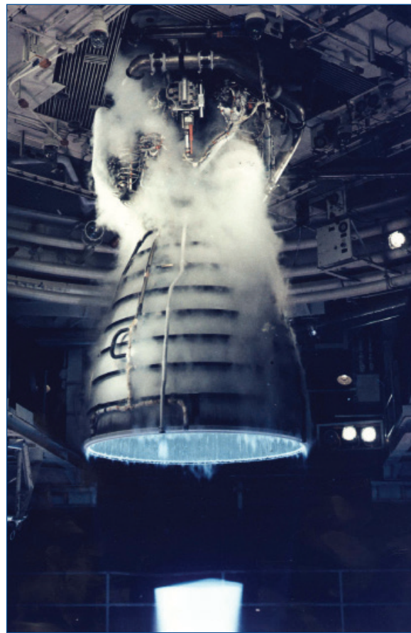
Space shuttle main engines test independently in the A Test Complex, simulating sea level (A-1) and high altitude (A-2) testing.
