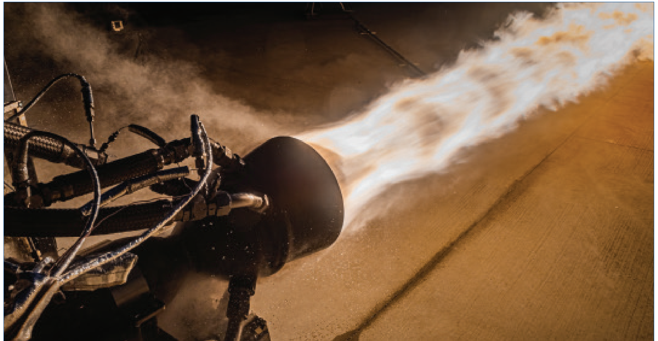
Launchers 3D-printed Engine-2 (E-2) rocket engine completes a 5-second hot fire Aug. 20 of its latest thrust chamber assembly. (Credit: Launcher / John Kraus Photography)
