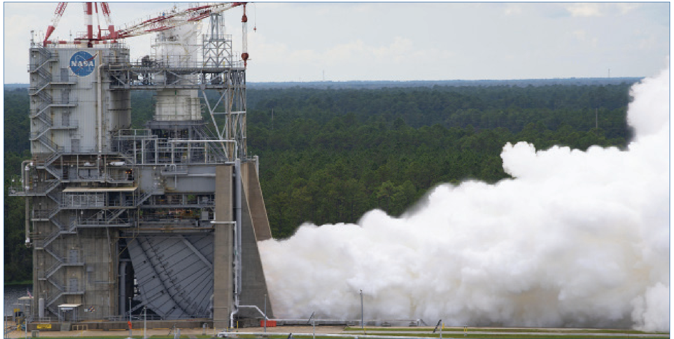
NASA conducts a full-duration RS-25 hot fire test on the A-1 Test Stand at Stennis Space Center on Sept. 30. The hot fire of more than 8 minutes marked the final test of a Retrofit-2 series.
