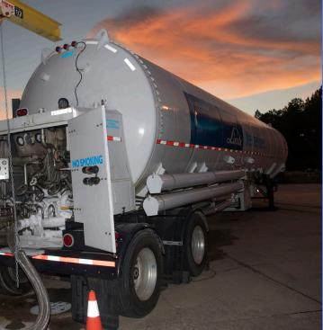
(Left photo) Heavy condensation early on the morning of Oct. 19 signals the transfer of super-cold liquid nitrogen into large vaporizers used to convert the liquid to a gaseous state at the Stennis Space Center high-pressure gas facility. Operators conducted a critical "stress test' of gas house capabilities Oct. 18-19 to demonstrate its readiness for upcoming
