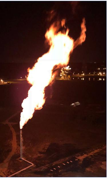
Liquid hydrogen is burned out through a flare stack at the B-2 Test Stand during a propellant cold flow test. The successful cold flow test marked a major milestone in activation of the stand for testing NASA's SLS core stage.
