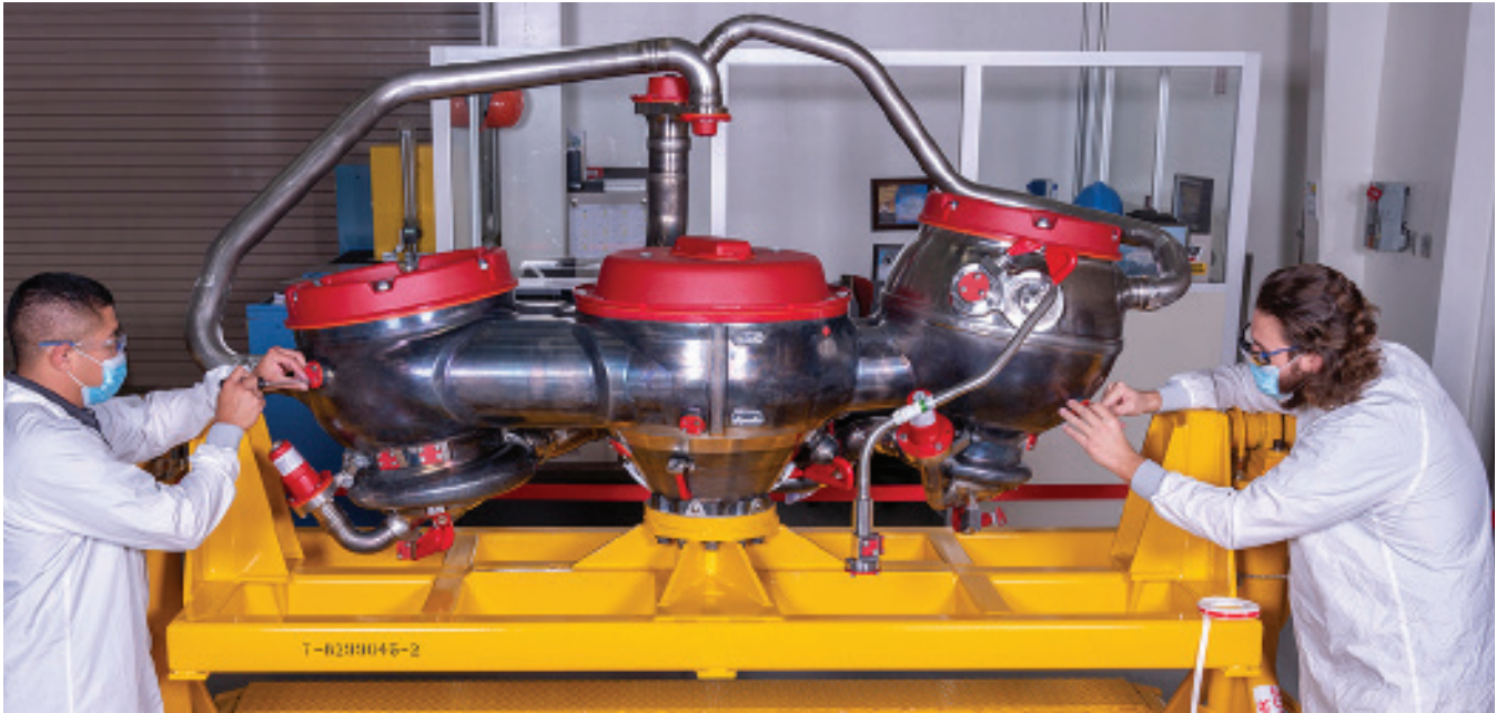
Two engineers look over an RS-25 powerhead that arrived at Stennis on Oct. 25, after it was pressure tested at Aerojet Rocketdyne's Los Angeles site.
