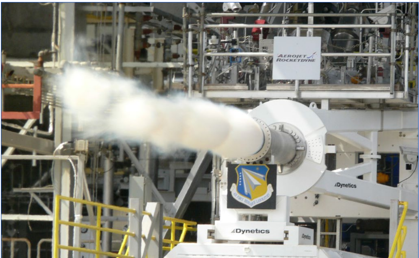
The Air Force Research Laboratory successfully tested a state-of-the-art rocket engine preburner on the E-1 Test Stand at Stennis to elevate the U.S. technology base for high performance oxygen-rich staged combustion, developed by Aerojet Rocketdyne. Testing at Stennis concluded Sept. 30.
