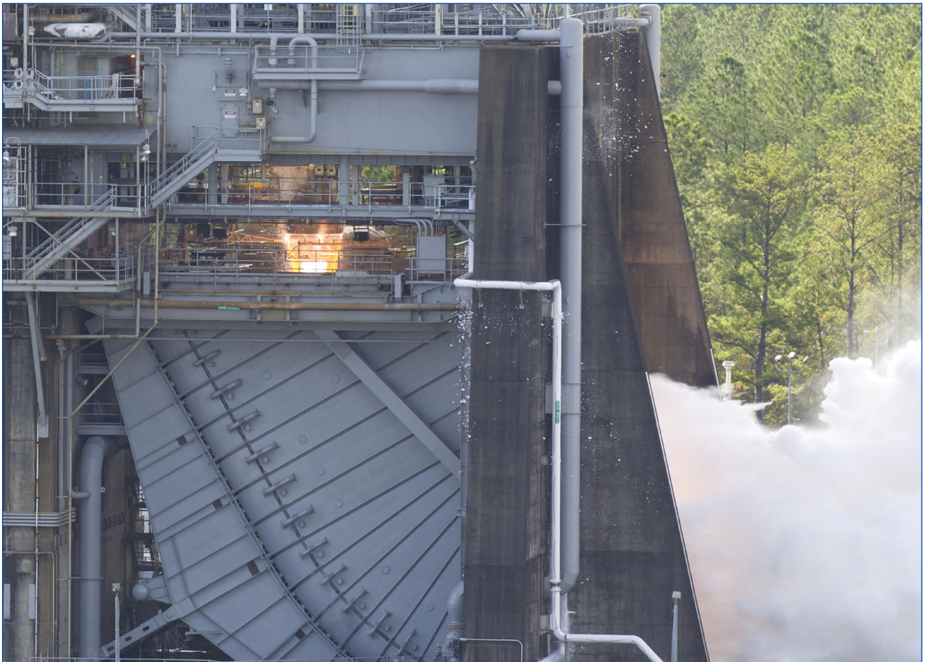
A zoom-lens photo captures the fire power of the RS-25 rocket engine as it is tested on Oct. 19 during Stennis Space Center Founders Day Open House.
