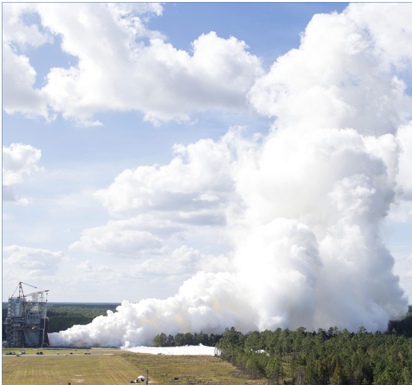
NASA engineers conduct a full-duration, 500-second test of RS-25 flight engine E2063 on the A-1 Test Stand at Stennis Space Center on Oct. 19, 2017. Once certified, the engine is scheduled to
