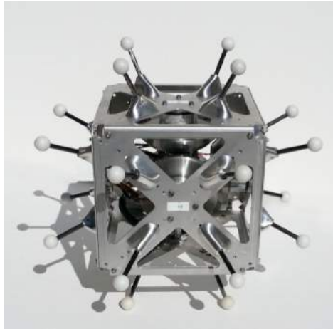
Figure III.5. Hedgehog prototype I (payload and solar panels not included) [Reid, R. et al. 2014]
