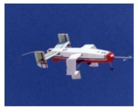
Figure 3-17: I2000, an airship with inflatable wings, successfully test in Earth's atmosphere [42].
