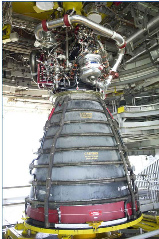
An RS-25 engine sits at the A-1 Test Stand at Stennis Space Center prior to complete installation and testing.
