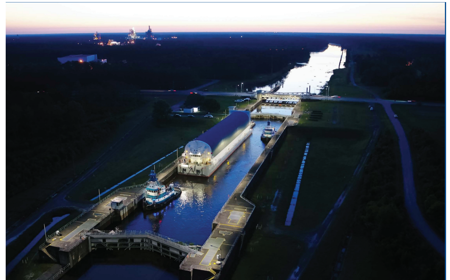
A drone photo shows NASA's Pegasus barge as it passes through the lock system at Stennis Space Center on April 23, 2021. The barge was beginning transport of the first Space Launch System core stage to Kennedy Space Center, following completion of a Green Run test series on the B-2 Test Stand (seen in background).
