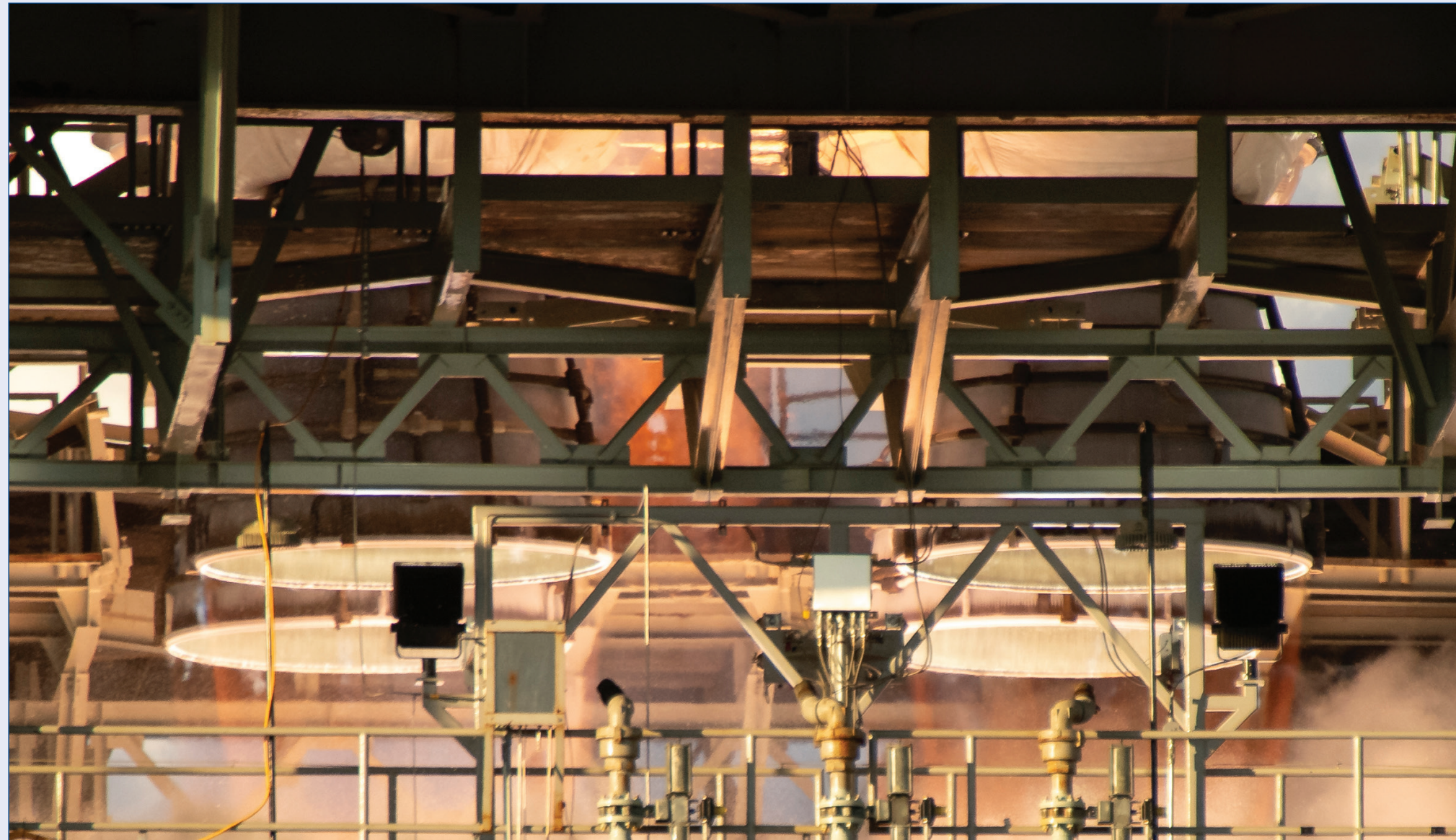
A close-up photo offers a view of four RS-25 engines firing simultaneously during the Green run hot fire test of NASA's Space Launch System core stage at Stennis Space Center on April 18, 2021. The hot fire test one year ago culminated a series of Green Run tests of the core stage and its sophisticated systems. The stage now is being readied to help launch the Artemis I mission to the Moon.
