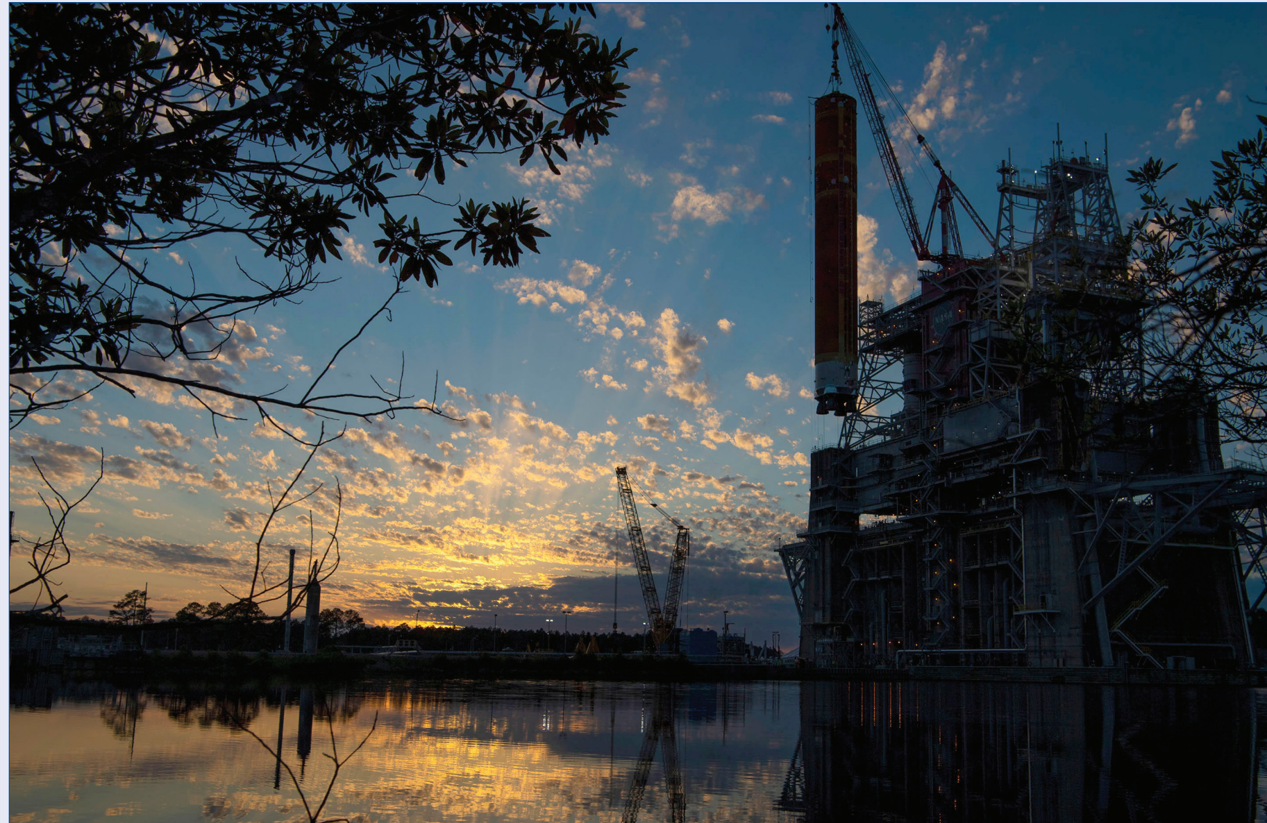
The first Space Launch System core stage hangs suspended from the B-2 Test Stand crane at Stennis space Center on the morning of April 20, 2021. Stennis teams removed the core stage during overnight operations before lowering to the test stand tarmac and loading it onto NASA’s Pegasus barge for transport to Kennedy Space Center. Removal of the stage followed completion of the Green Run series of tests on the stage and its integrated systems. The stage now is being readied for the upcoming launch of the Artemis I mission to the Moon. Photo Credit: (NASA/Danny Nowlin)
