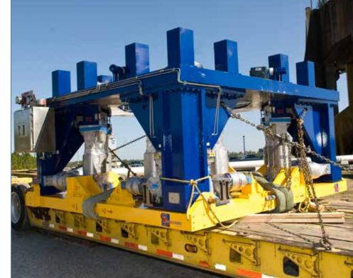
A state-of-the-art thrust measurement system arrives at the A-1 Test Stand for installation in 2010. The system is a precisely calibrated component used to collect thrust data during a rocket engine test.
