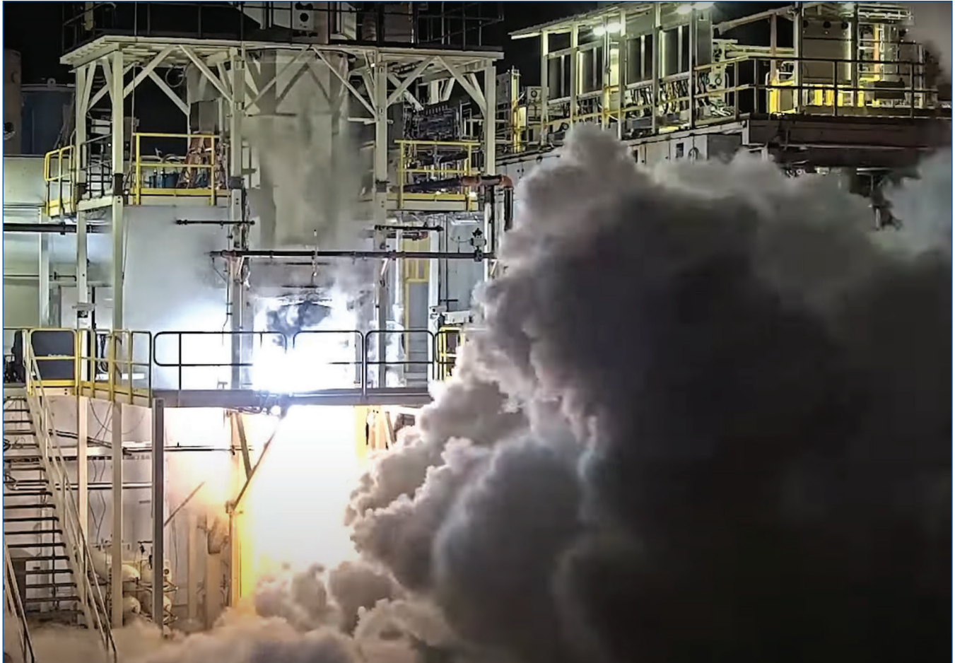
Relativity Space Inc. conducts a mid-May hot fire test of its Terran 1 second stage on the E-4 Test Stand at Stennis Space Center.
