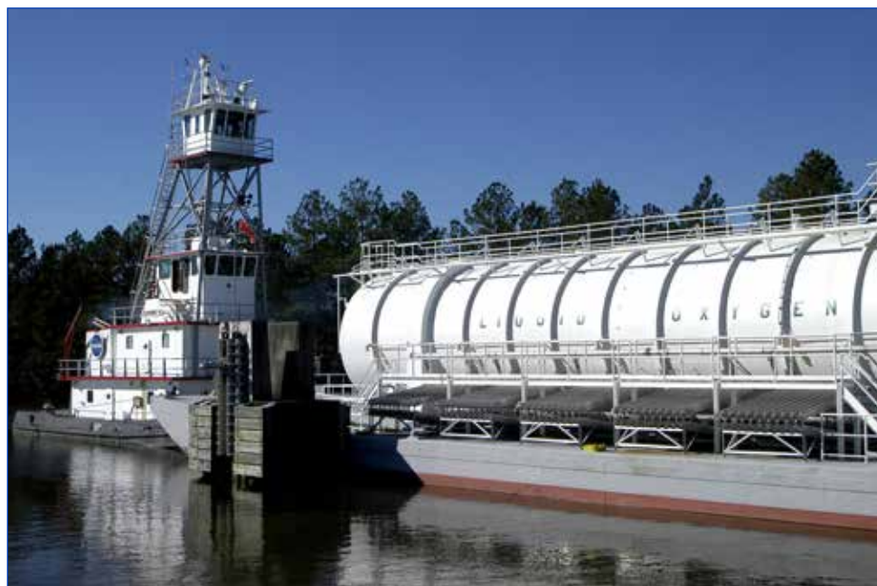
A liquid oxygen tank barge is delivered to a Stennis test stand to support rocket engine testing.
